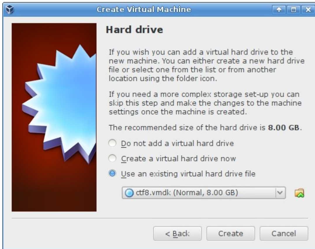
Illustration 4: Specify the existing virtual machine hard drive.
